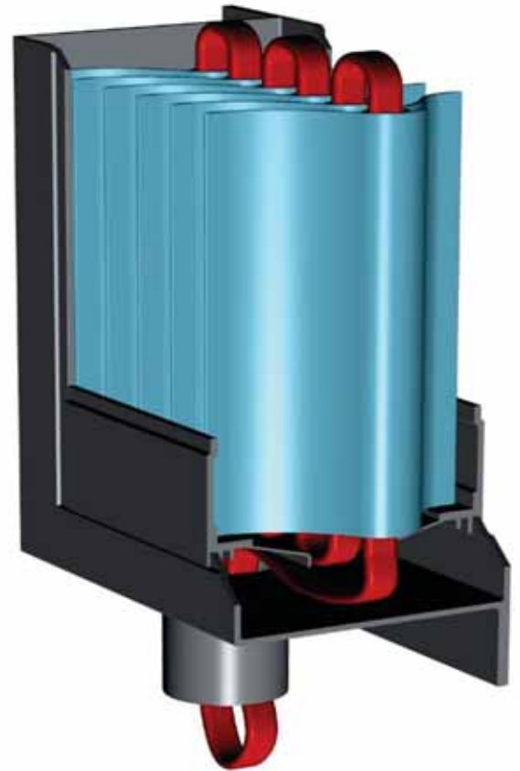
Figure above illustrates how the heating cable is routed through the vanes and out of drain pipes.
